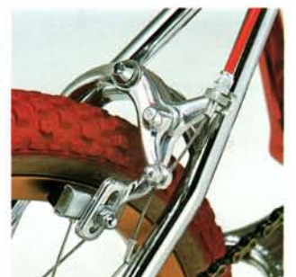
BRIDGESTONE's own patented SC (Self-Centering) brake with AW Brake Pads
