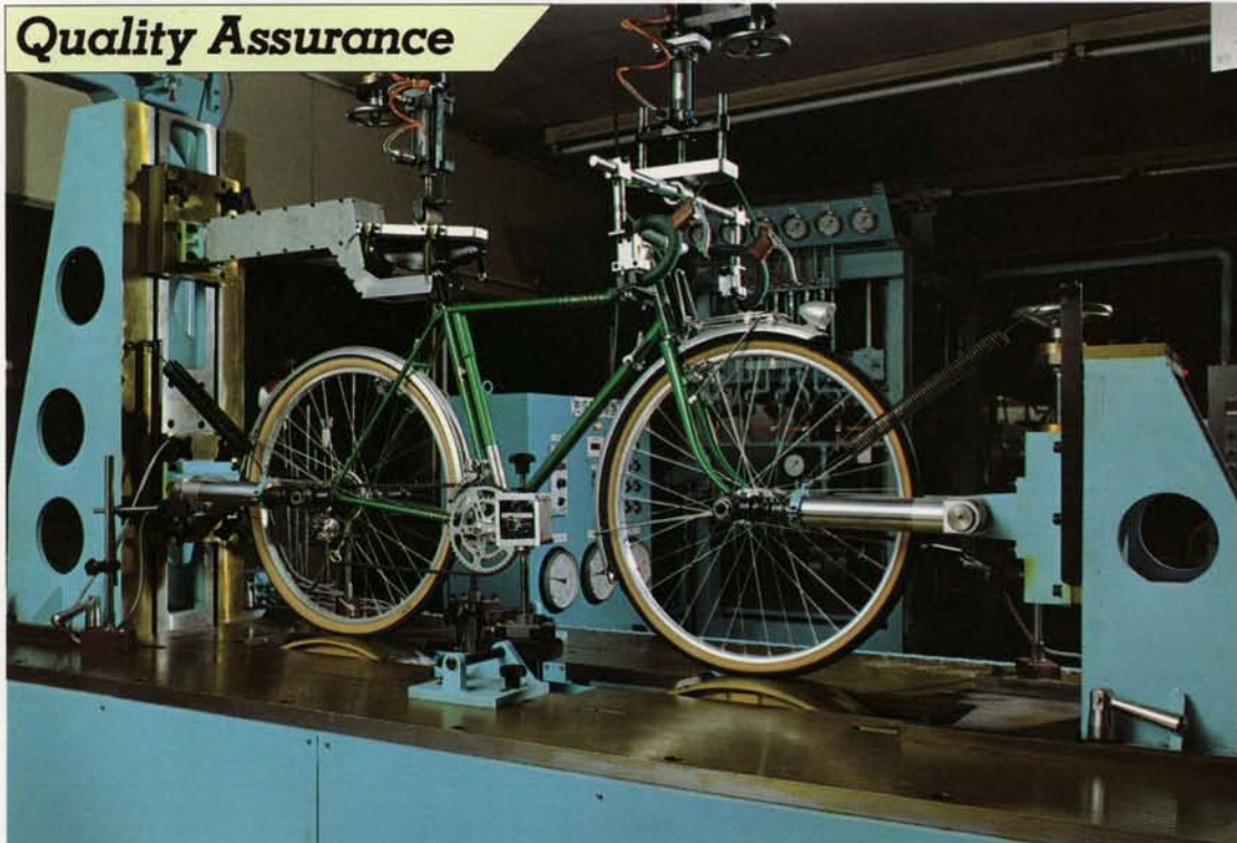
Final endurance test machine.
